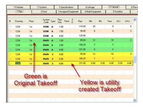
The yellow pipe sizes are the OD of the insulation from the green pipe sizes.
